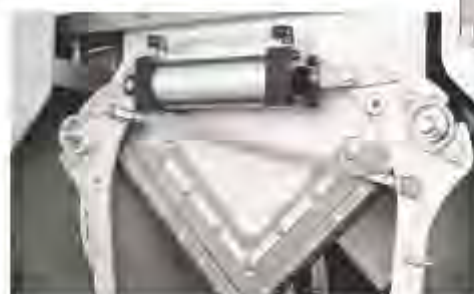
Stainless steel gravity gate and weigh bucket, with hydraulic hinge
